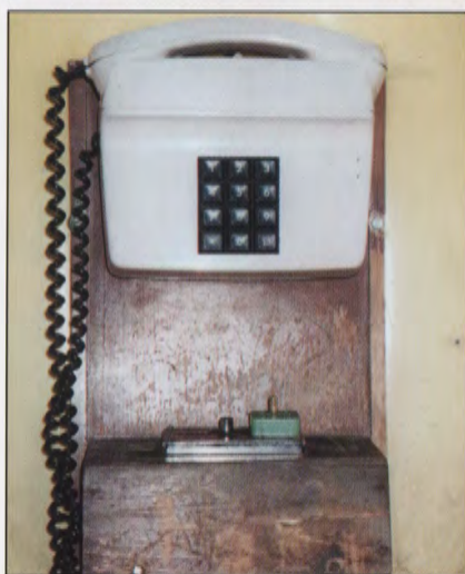
At first glance you might think this wasn't a payphone at all. You'd be wrong. Found by a Ghazian gas station, this phone has a slide coin chamber which would last about 30 seconds in the States.
