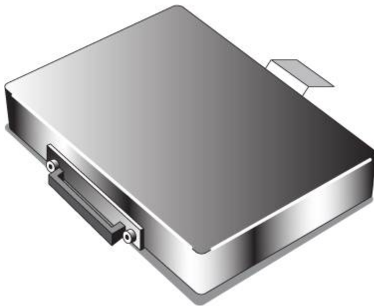
Figure 9.4. Hard drive caddy used in ThinkPad 770 laptops.
