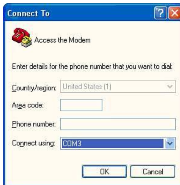
Figure 12.8. The HyperTerminal dialog box showing how to access a particular COM port.
