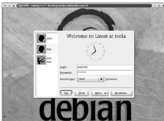
Figure 26.8: Linking VNC to XDMCP gives you a traditional Linux GUI login over VNC.
