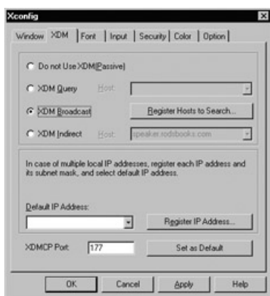
Figure 26.3: Windows X servers typically provide a GUI tool for setting XDMCP server options.
