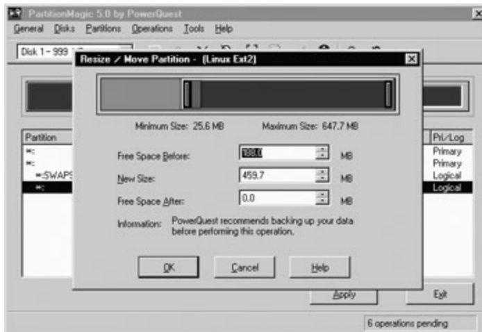
Figure 10.1: PartitionMagic provides a GUI interface to simplify partition resizing.
