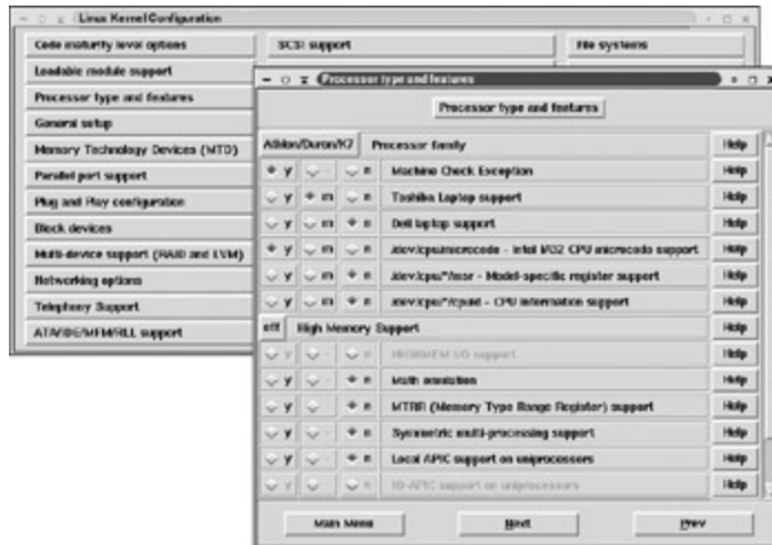
Figure 15.2: The make xconfig kernel configuration command presents a GUI menuing system for selecting options.
