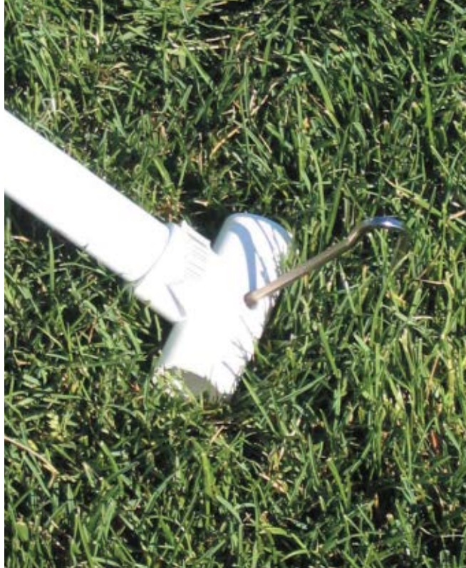
site, thread a tent stake through the holes in the T-junctions and press into the ground.
