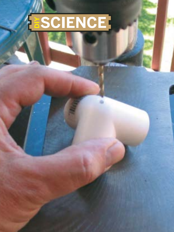
Drill a hole down the center of the corner junction's rounded "elbow" for different launch rods. At the launch
