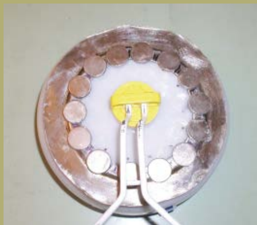
Magnet wheel assembly attached to side of rodent exercise wheel.
