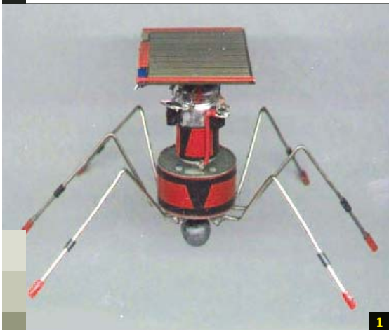
1 Jim Mullins' Symet3-Virus, which is basically a Type 1 (voltage-triggered) Solarengine with an added ball-tip "motivator" on the motor shaft and a set of six legs, upon which this robotic top can skitter around.
