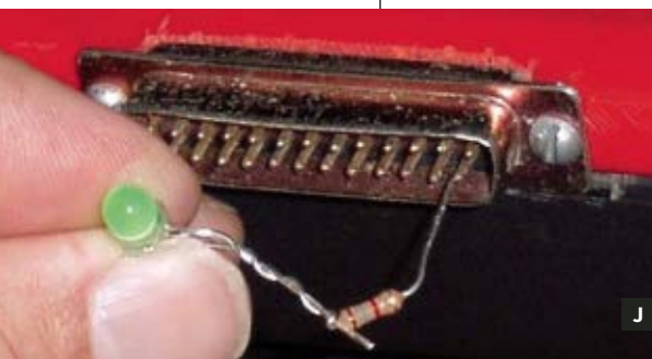
Fig. H: The matrix tester is made from an LED and a 1k resistor. Fig. I: Use this circuit to determine the polarity of the phototransistor. Fig. J: Attach the resistor to the ground pin and touch the LED anode to each pin,
