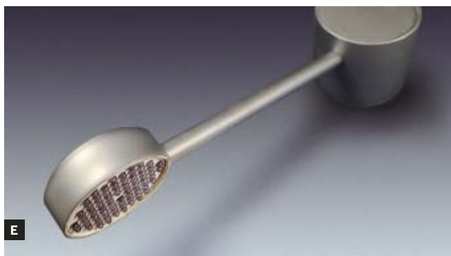
glued into a 1" hole in the head. Fig. D: The mounting plate is ABS plastic drilled with 72 holes. Fig. E: The finished lamp, with the head tilted to show the LEDs. Total cost: about $40; total power consumption: about 5W.
