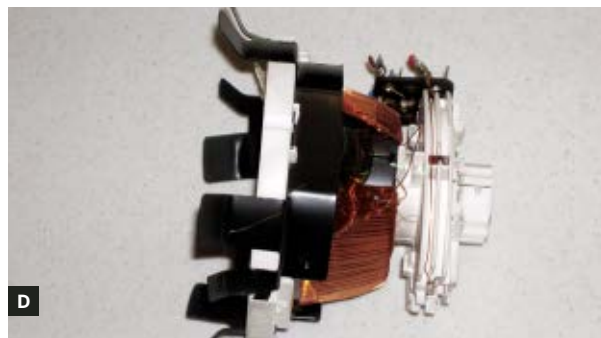
Fig. C: Colpitts oscillator circuit uses TV components to generate a sine wave you use as a broadcast carrier. Fig. D: The flyback transformer, which pulls the tube's beam along its scan pattern, has lots of winding wire.
