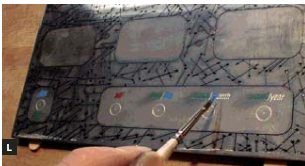
Fig. K: Filling in the etched arrow details with a fine paintbrush and black enamel paint. Fig. L: Filling in the color detail with more enamel.
