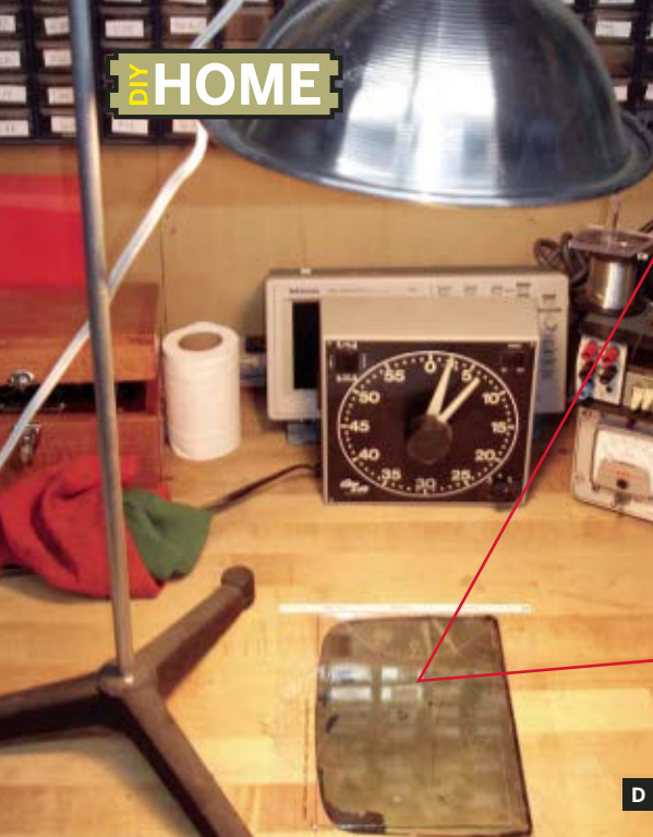
Fig. D: Expose the coated metal plate for 4 minutes under a 500W photoflood lamp, with the reflector positioned 18" above. Don't worry if the reflector isn't rated for a bulb that hot; it isn't on for long enough to matter.
