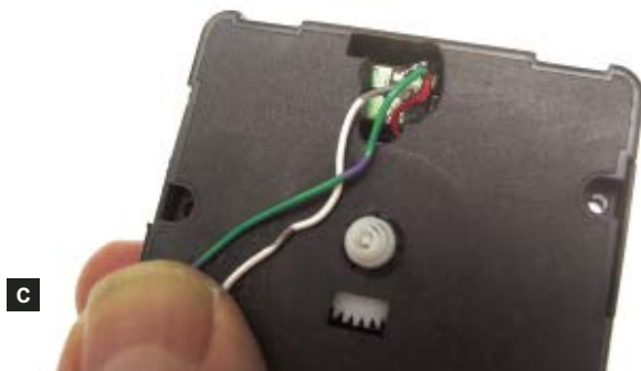
Fig. C: New wires to your own circuit connect to the electromagnet through the clearance hole in the now-bare clock face.
