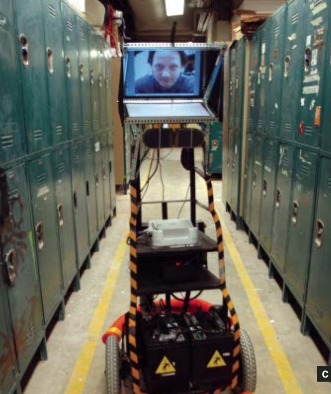
Fig. C: Marque Cornblatt's Sparky 2 projects its user's presence anywhere the robot can find a wi-fi connection. Fig. D: The Bovalve controller combines the concepts of a violin bow and trumpet valve system to play a
