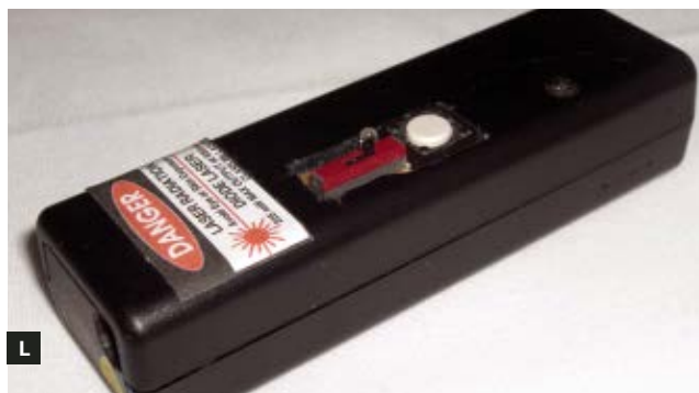
Fig. K: Laser, circuitry, and batteries hot-glued into plastic enclosure. Fig. L: The finished, pocket-sized high-power laser.
