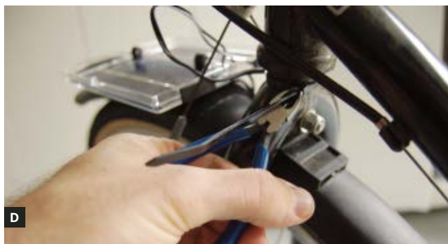
Fig. C: Bolt a car dashboard PDA holder to the handlebar, then Velcro the PDA in there. Fig. D: Tuck the wires away with cable ties, and you're rolling.
