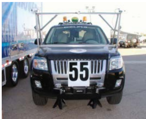
LOW BUDGET: Mahesh Chengalva wrote all the code for the low-budget, high-ambition Ody-Era (#55). Other robot cars had so much computer power that they required onboard gen-sets for power and air conditioning.
