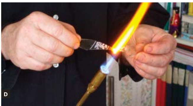
Fig. C: The wiring on the underside of the lid for the fan motor control and stylus. Fig. D: Glass thread is pulled from shards to make the stylus.
