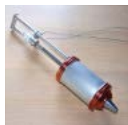
CLOCKWISE FROM LEFT: The Fab@Home extruder is a syringe driven by a linear actuator; the Stratasys Dimension 3D printer extrudes a filament of heated plastic; the author's DIY cookie press, retrofitted for computer control with a $6 motor.
