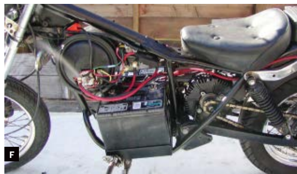
motor, bolted to the mounting bracket on the swing arm. Fig. F: The GomiCycle's wiring, on an earlier version of the bike, with 80Ah batteries. We stuffed the electrical components into a camping cooking pot.
