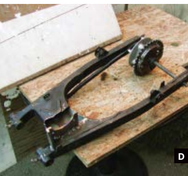
Fig. B: The original, overbuilt battery tray for the engine compartment. Fig. C: The stripped motorcycle frame. Fig. D: The swing arm, with a clearance hole and mounting bracket for the motor. Fig. E: The electric
