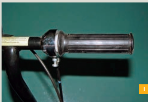
Fig. D: Rear axle and brake moved back on the swing arm to accommodate a larger rear wheel. Fig. E: Right-angle gearbox mounted to a custom tapped plate that's screwed to the original motor mount. Fig. F: Aligning the sprockets. Fig. G: Wooden kickstand extension. Fig. H: Gearbox shaft milled into a triangular shape, for a stronger hold from the drill chuck. Fig. I: Handlebar twist-grip for throttle cable. Fig. J: Throttle mechanism, cable side.
