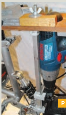
Fig. K: Drill trigger side of throttle mechanism, showing lever rounded at the contact point. Fig. L: Rear wheel shock absorber. Fig. M: Hinged slip-joint connection between the drill support platform and the seat post. Fig. N: Support plate with hook for holding bottom end of the drill. Fig. O: Back end of drill, shown being steadied by the swing arm. Fig. P: Support pillar between the main support platform and the gearbox mounting plate. Fig. Q: Bracket securing the bottom end of the support pillar. Fig. R: Completed Drill Rod, in all its glory, equipped with a spare battery pack in the frame.
