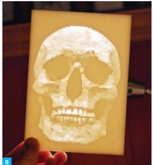
Fig A: My micRo CNC robot, built from a kit. It was easy. Fig. B: The bot milled this plastic to different depths, using a simple CAM program.
